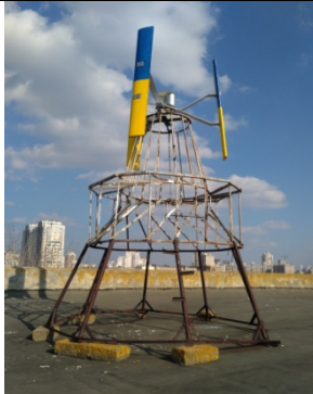
Fig. 3. Experimental sample of designed VAWT rotor
