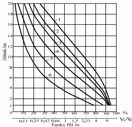
Fig. 2. Theoretical dependence of oxygen concentration in the space above fuel from the volume of the tank filled with fuel and altitude of an aircraft: 1 -  $O_2$  - 33 %; 2 -  $O_2$  - 29 %; 3 -  $O_2$  - 27 %; 4 -  $O_2$  - 25 %; 5 -  $O_2$  - 23%; 6 -  $O_2$  - 22 %
