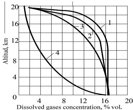
Fig. 1. Dependence of the dissolved air amount in the RT fuel, altitude and aircraft rate of climb ( $V_y$ ): 1 -  $V_y=75$  m/s; 2 -  $V_y=45$  m/s; 3 -  $V_y=15$  m/s; 4 – according the Henry's law.
