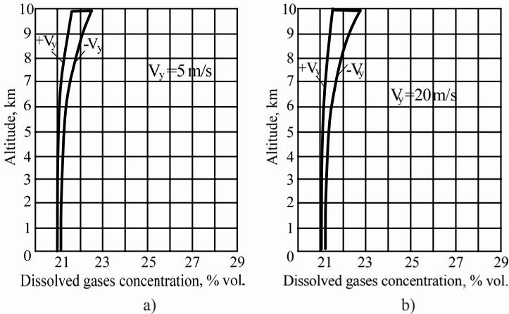
Fig. 3. Change of oxygen concentration in the space above fuel as the tank is risen to the altitude and at 20 % fuel tank filling
