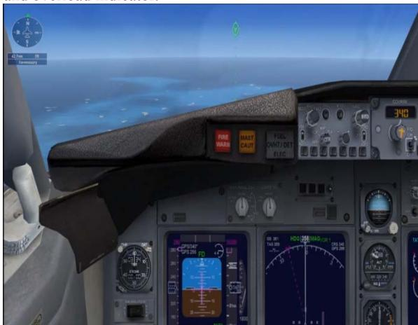
Fig. 2. Attack angle indicators in the cockpit of Boeing 737
