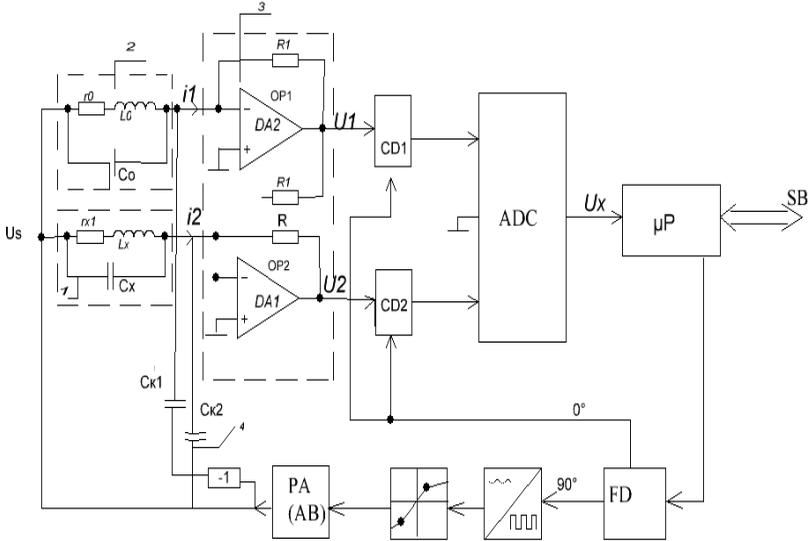
Fig.1 Functional scheme of the measuring channel.
