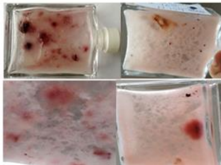
Figure 1. Microbiological damage to jet fuels.
