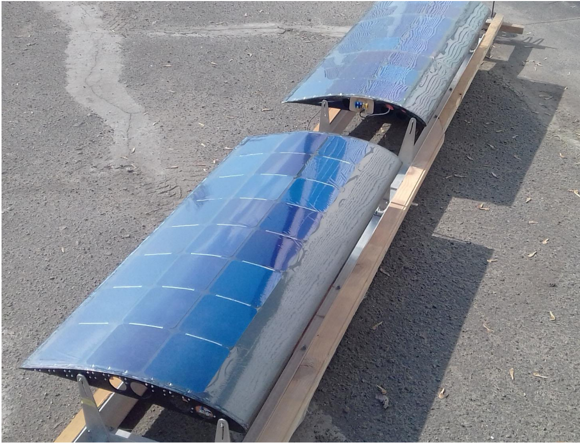
Figure 2. Solar cells battery at the surface of experimental section of the wing.
