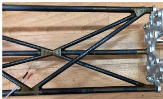
Figure 14. Connection of upper and lower rods with braces and end frame of tail beam by means of aramid thread
