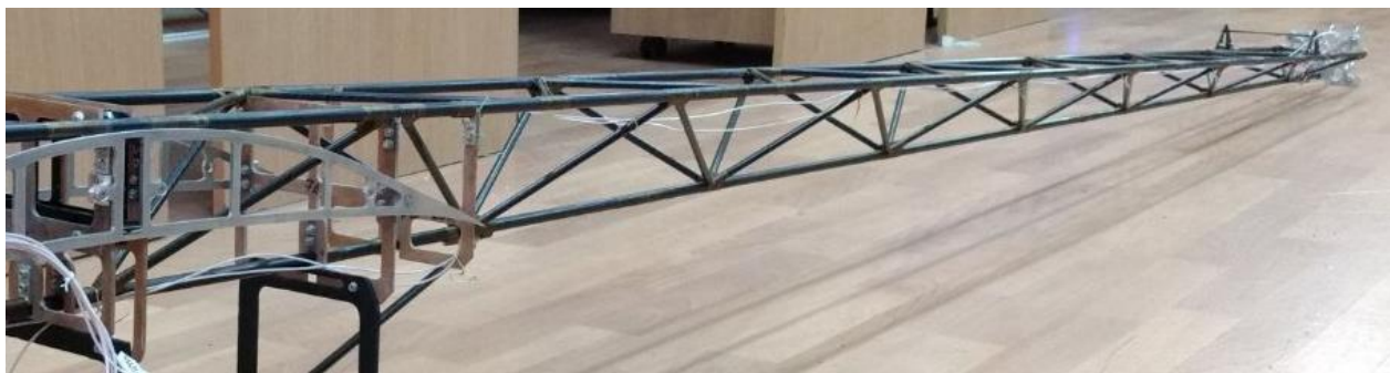
Figure 9. Appearance of the main components of the tail beam of the pseudo-satellite
