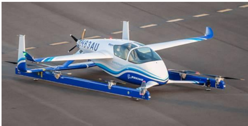
Figure 7. Aurora's electric vertical take-off and landing (eVTOL) aircraft PAV prototype. Source: http://www.aurora.aero/pav-evtol-passenger-air-vehicle/
